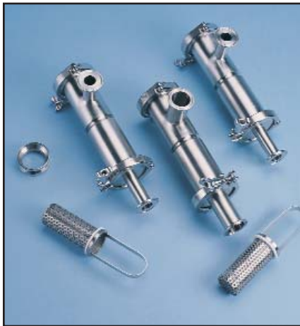
Basket Strainer-Model S10 (325 mesh lined baskets)
